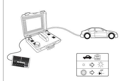
The Lightmate 3 simulates the electrical current load (Amps) on the individual lighting circuits so that the correct operation of the socket functions and any electronics can be checked.
