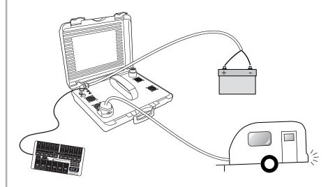
With the use of an external 12V battery you can power the individual road lighting circuits on a trailer or caravan.
